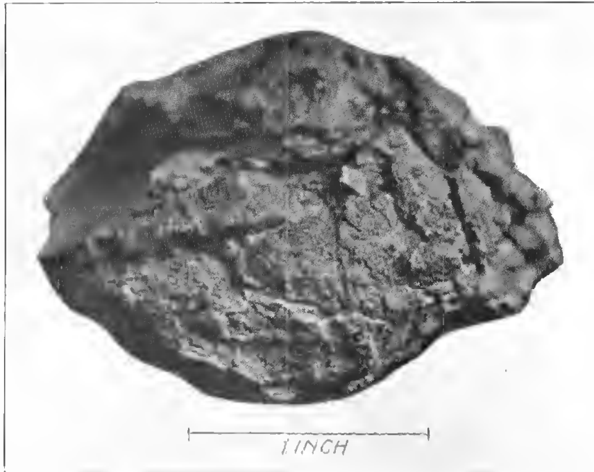
Fig. 9. "Iron-shale" showing typical bi-convex shape.
